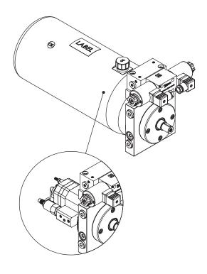
The W84BT series power pack is designed for applications that need high pressure and larger flow, but use a customer supplied low-power transmission. Because the power pack uses a standard manifold (W800532), they will have the same functions as the W80BT series power pack.
